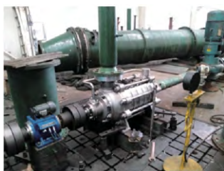
图6 HSB220/620 海水淡化高压泵测试装置 Fig. 6 Test rig for HSB220/620 seawater desalination high pressure pump
